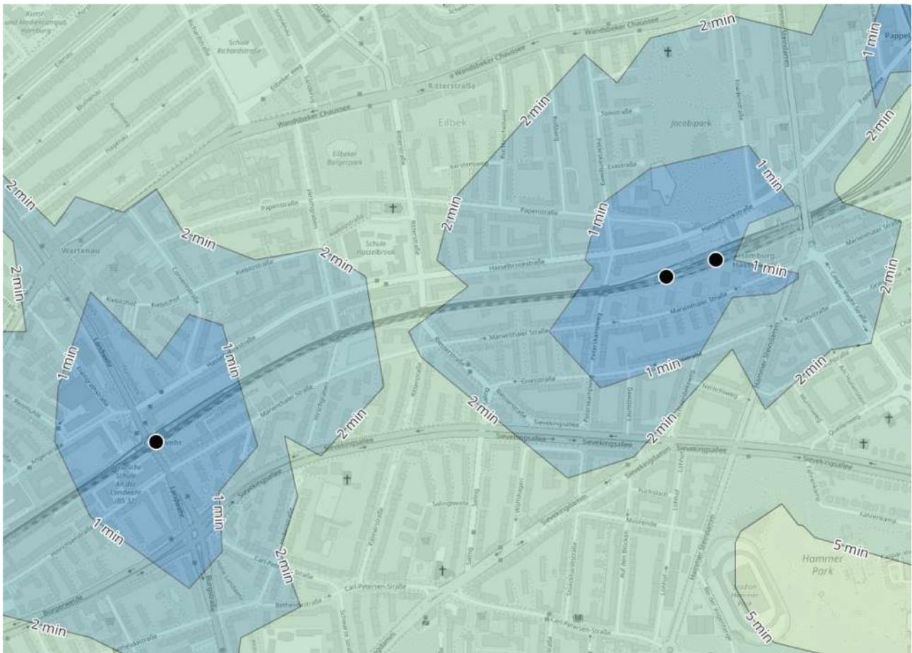
Figure 4: Example on using bikeable links in OSM to calculate cycling time to nearest train station in GIS (Source: Data from OSM)
