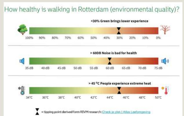
Figure 19: Overview of tipping points of when a street becomes “unhealthy” for pedestrians based on parameters such as greenery, noise, and temperature. Credit: City of Rotterdam
