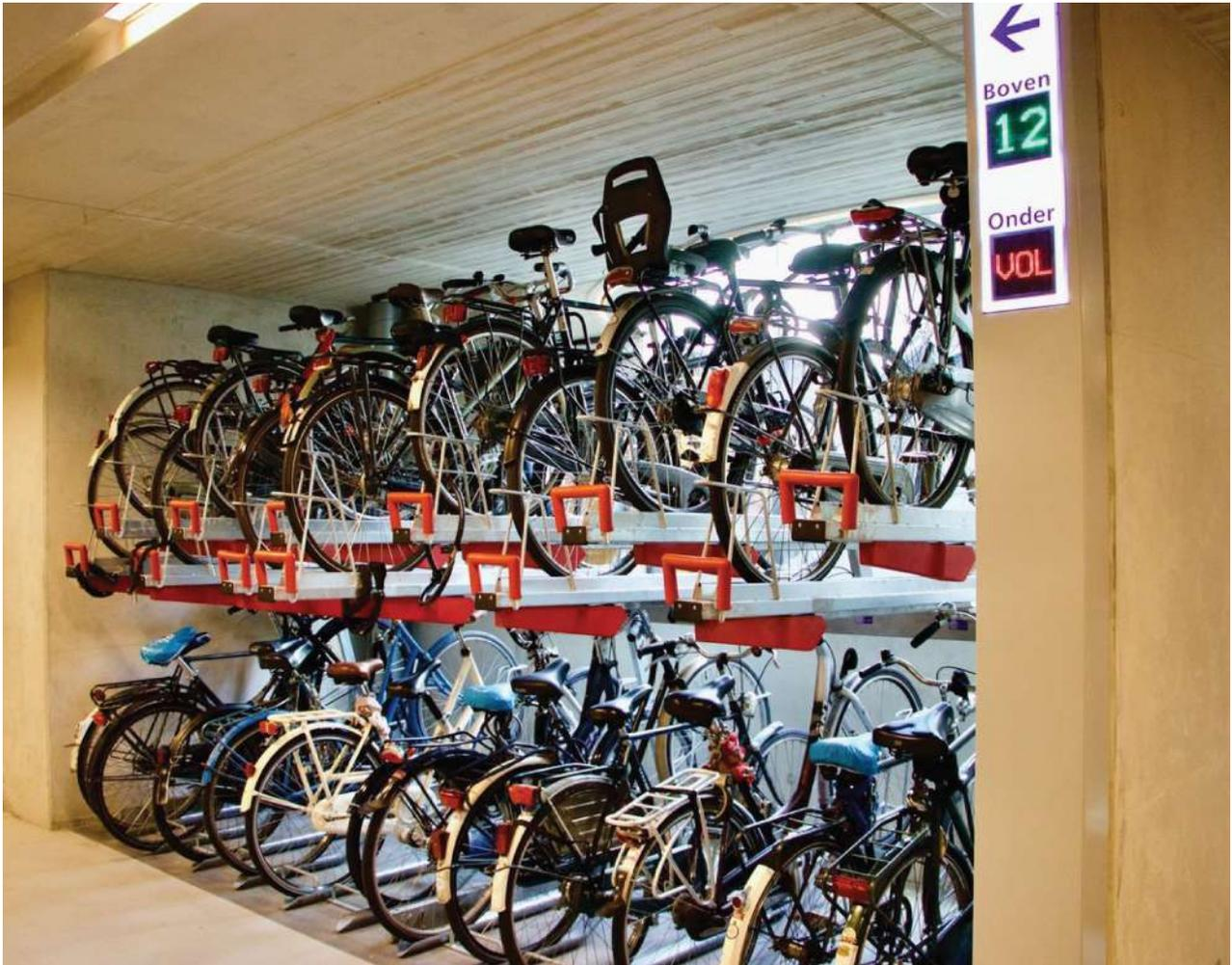
Figure 17: The Utrecht Stationsstalling with automated data collection and electric light signs to indicate vacant spaces (Source: <https://www.welovecycling.com/wide/2019/09/30/worlds-biggest-cycling-garage-opens-obviously-in-the-netherlands/>)
