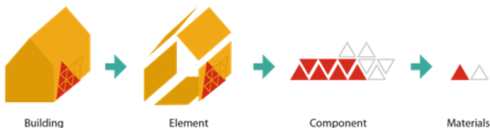
Figure 4: Hierarchical structure of the MMG method and SLiCE model
